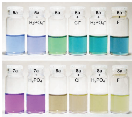
Figure 1. Colour changes of ligands in \text{CH}_2\text{Cl}_2 in the presence of anions (3 equiv of TBA salts).
